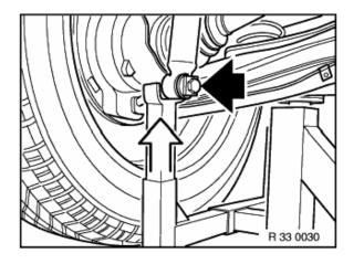
Slightly raise semi-trailing arm, unfasten screw, remove shock absorber and lower semi-trailing arm slightly.
