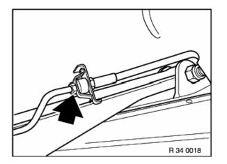
Disconnect left and right brake pipes.
